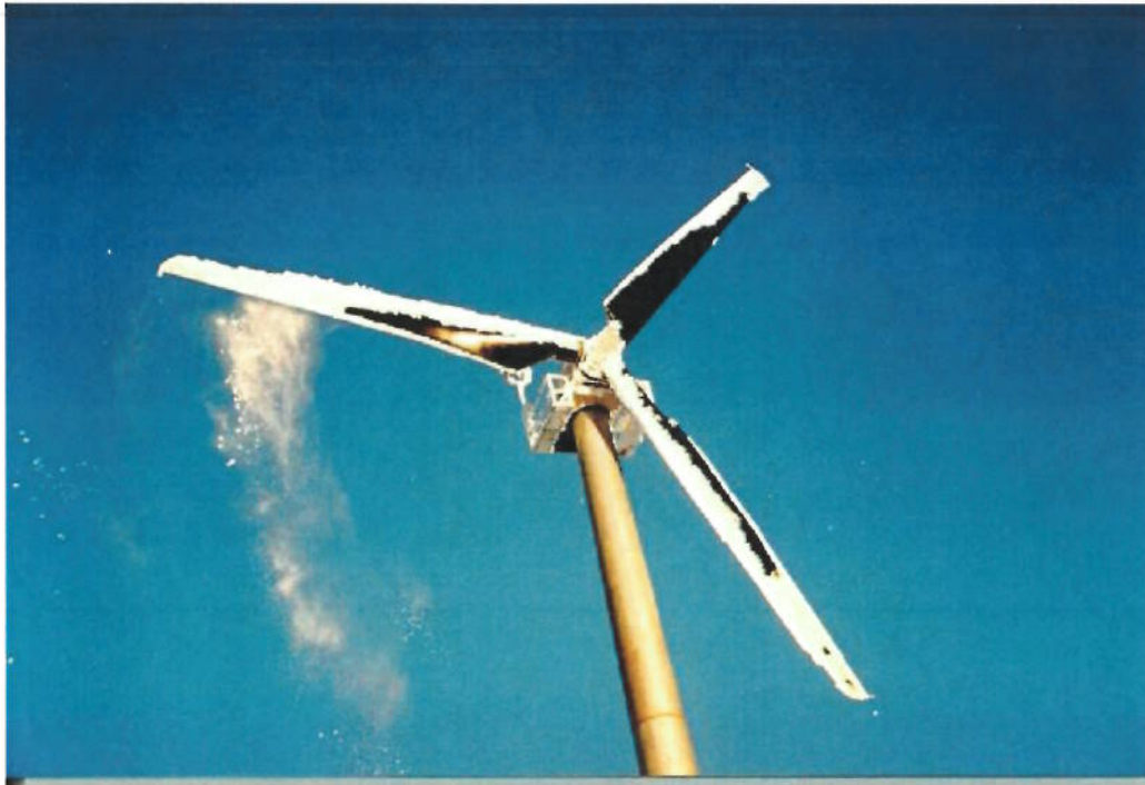
Photograph 8: accumulated ice shedding from black blades
