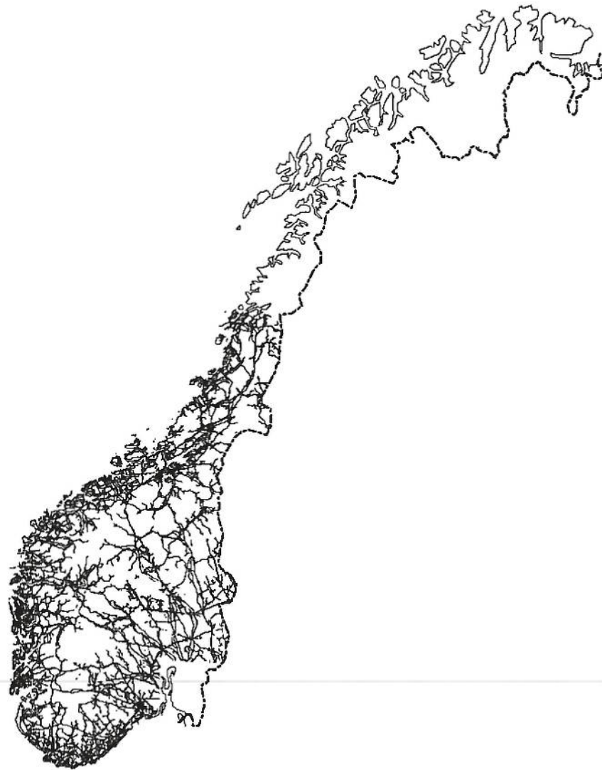
Fig. 1. Digitized data for the geographical distribution of high tension power lines (11–420 kV) in Norway. There are insufficient data for the three northernmost counties, Nordland, Troms and Finnmark and the three counties in the south-east — Vestfold, Østfold and Akershus. Data provided by the Defence Mapping Agency.
