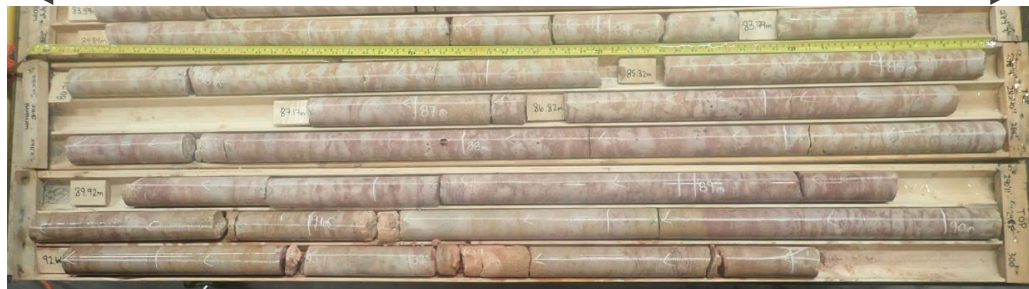
Figure 6: Image of collected cores for logging borehole DEN 117-1
