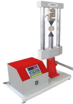
Figure 7: Point Load Test
