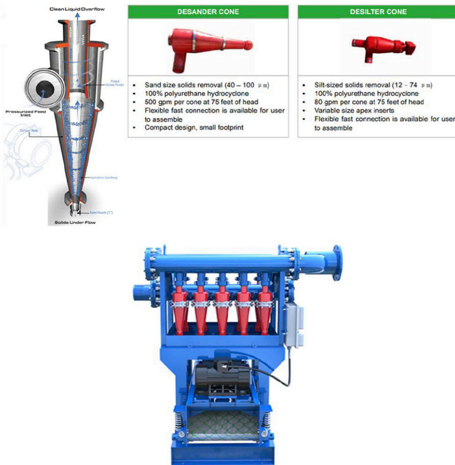
Figure 4-2: VorSpin Hydrocyclone (top) and KOSUN Desilter System (below)
