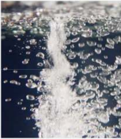
Fig. 6. Formation of vortex due to plunging jet ( v_N = 3.2 m/s, d_N = 4 mm, H_N = 300 mm)
