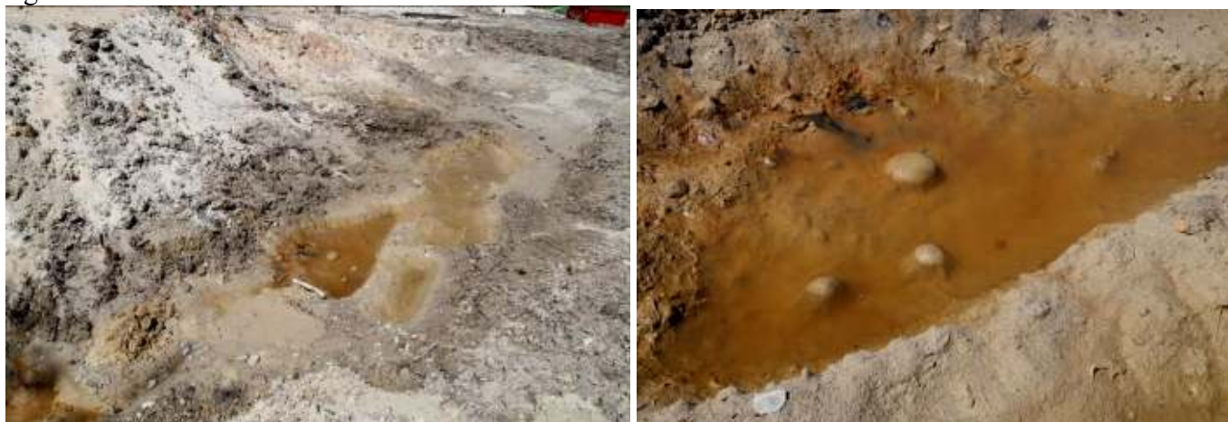
Figure 31. Sio Silica extracted sand pile near Vivian showing yellow/orange gelatinous deposits Image was used with permission of the photographer.
